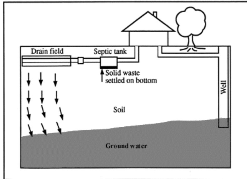
For a leaching system to function properly it must:
